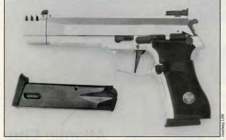
SP1 Sport Nickel Tuned model features an electroless nickel finish slide with the aluminum frame "natural" anodized. This model has a muzzle compensator. The high-profile front sight is pinned to the muzzle compensator to increase the sight radius. It also features an Italian LPA adjustable rear sight.
